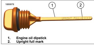
Figure 1. Engine Oil Dipstick
