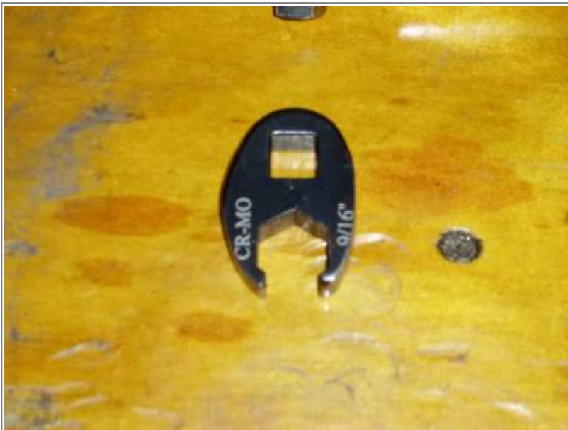
Crows foot for the 9/16" base nut. If you grind down a crows foot like this, it works quite well, 1)
