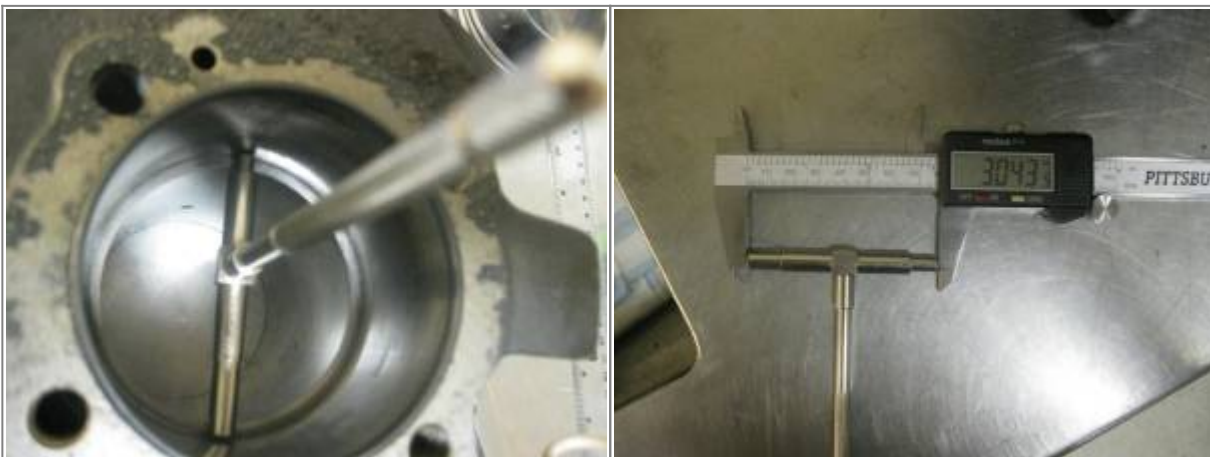
Telescoping bore gauge and caliper for measuring cylinder I/D. 2)
