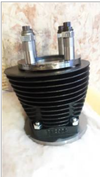
Torque plates installed. 4)
