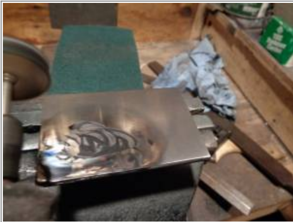
Too much compound 15)
