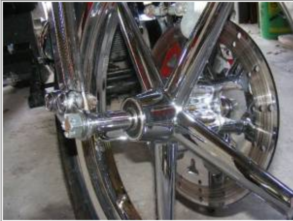
Polished stainless steel axle spacers 37)
