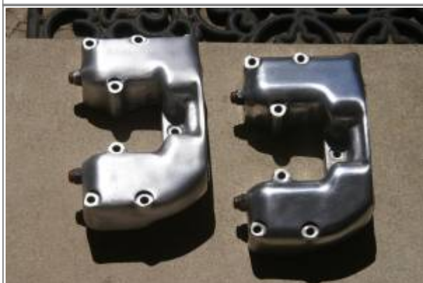
Ultra fine Scotchbrite on one side, followed by aluminum polish on the other: 30)
