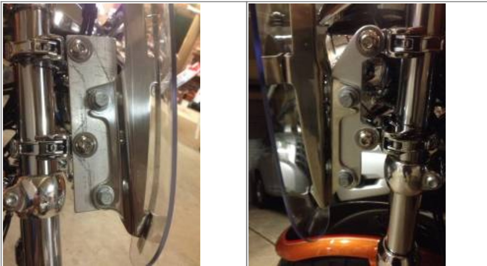
Homemade windshield lowering brackets with a polished brushed finish. 38)
