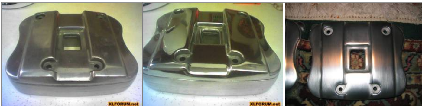
After much scotch wheel, dry & wet sanding, Scotchbrite and steel wool 29)
