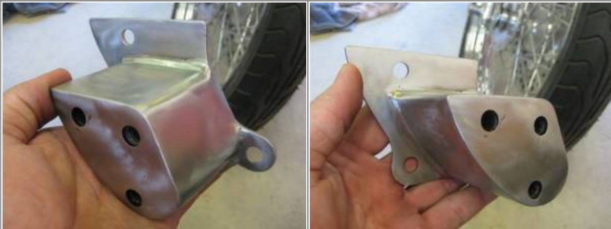
Custom made mounts to adapt BT forwards to a 77 model. 2)
