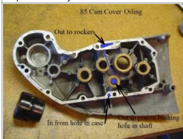
Oil path of 85 style cam cover 3)
