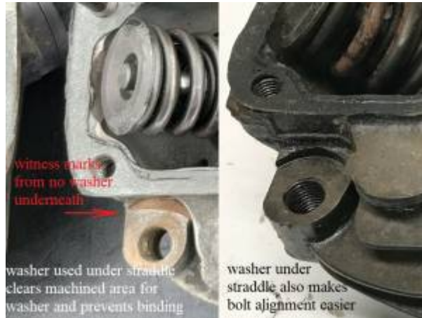
1960 XLCH Top Motor Mount (washer under head strap at each bolt, no washer under bolt head)
