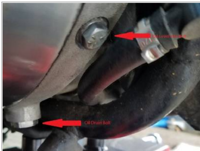
Primary / Transmission oil drain plug on 2001 Sportster 5)
