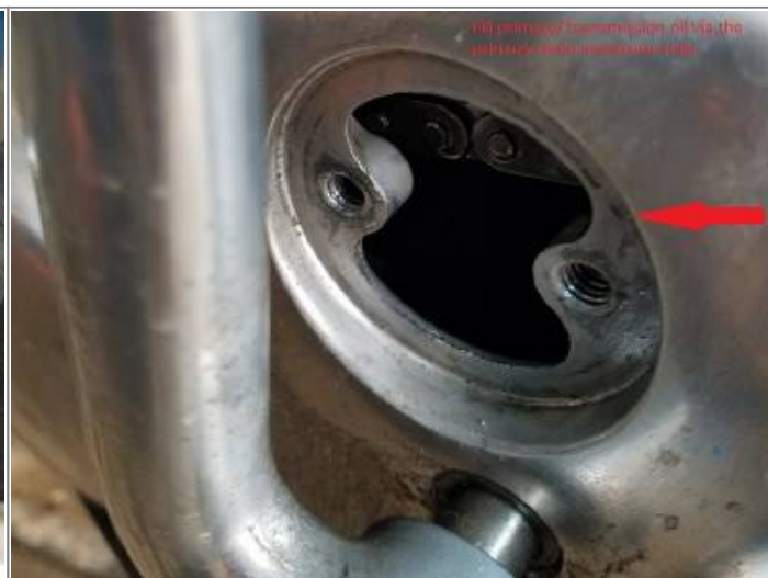
Primary / Transmission fill and check site for a typical 1994-later Sportster (1994 example) 6)
