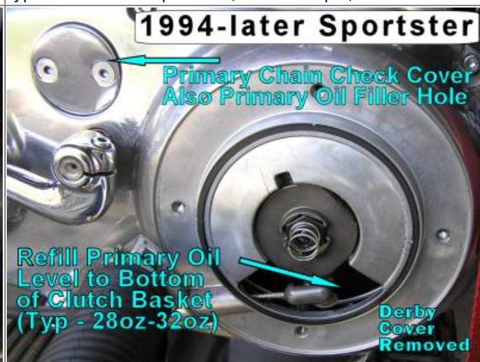
Primary / Transmission fill and check site for a typical 1994-later Sportster (1994 example) 6)
